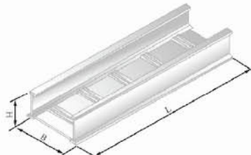
LQJ-01CP 型铝镁合金托盘桥架 Type LQJ-01CP Al alloy tray type cable support
